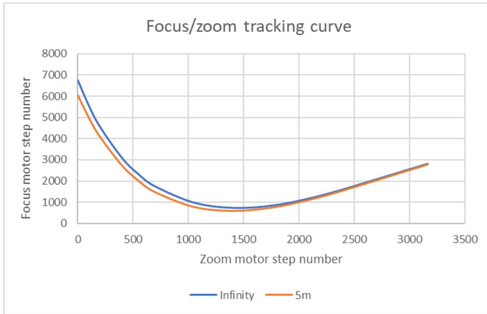
Fig 2.1: focus/zoom curve for 2 object distances for Theia's TL1250 calibrated lens.
