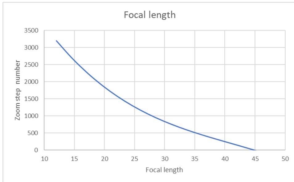
Fig. 2.2 inverse focal length calibration curve for Theia's TL1250 calibrated lens.
