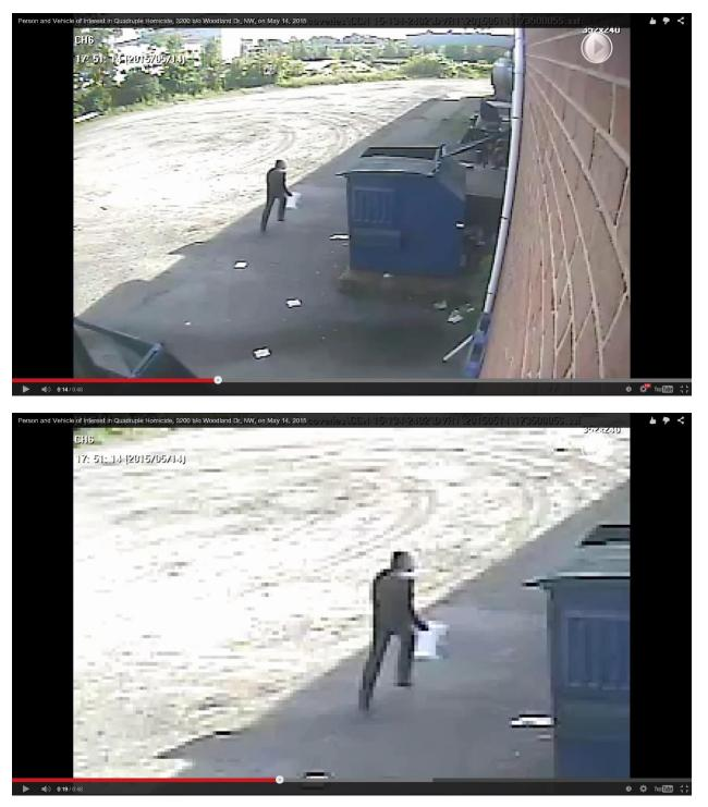
Although we don't know the exact details, we could assume from looking at the images, that the camera is approximately 10 metres away from the subject and the lens is about an 80 degree Horizontal Field Of View (HFOV) lens on a 1/3" sensor CIF camera. In that case, the pixel density in the image is only 21 pixels per metre, roughly 10 times less than the EN standard of 250 pixels per metre needed for facial
