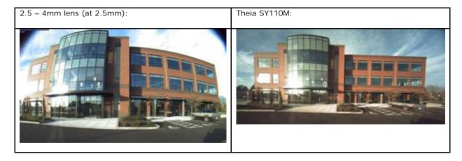
Theia's lenses correct barrel distortion in the optics of the lens without the use of de-warping software for a faster, real time solution. Image information lost due to the barrel distortion of typical wide angle lenses cannot be recovered even with the use of de-warping software.
