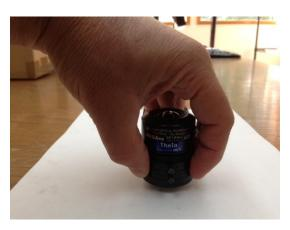
The <u>Not correct hand</u> picture shows the hand grab position that could damage the lens focus if too much downward pressure is applied.
