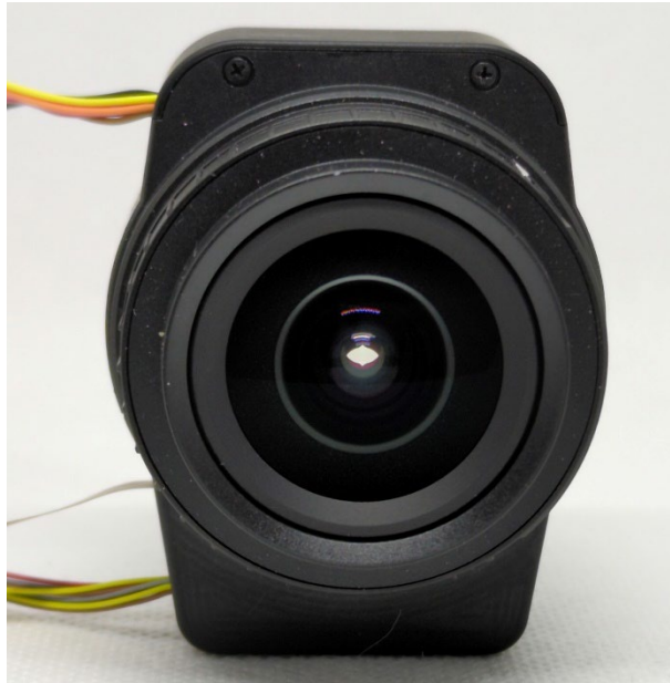
Fig. 1.2: aperture orientation in Theia's TL410 lenses
