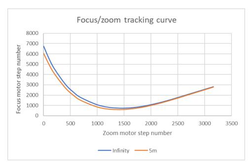
Fig 2.1: focus/zoom curve for 2 object distances for Theia's TL1250 calibrated lens.
